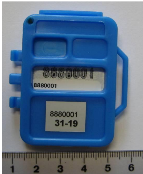
Figure 2. Example of a dosimeter with the label added by the coordinator. "8880001" is the identification code as provided by the participant. "31" is the code to identify the dosimetry system (note: for presentation of the results, a different code was used). "19" is the code to identify a specific radiation quality, angle and dose range combination from the irradiation plan.
